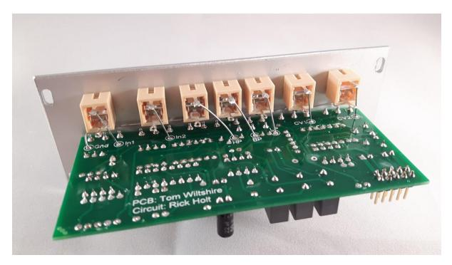
This is how I ground all the sockets to the PCB, The wire far left goes through the PCB ground pad:
