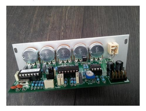
Image showing connection of (left to right): socket ground tabs, Bipolar out, Invert out, Normal out, Gate in, Mode switch, LED, Lin/Exp switch.
