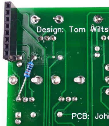
Instead do this with a 10K resistor.
