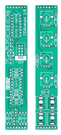
CEMvelope is based on the legendary ADSR section of the Sequential Circuits Pro-One monosynth, with minor adaptations to integrate it into Euro format. Smooth and snappy! It has a gate input as well as a trigger input, the trigger input works in conjunction with the gate input for multiple triggering from a suitable controller device. CEMvelope has at it's heart a CEM3310 or AS3310. You can source your own chip, of buy direct from me when you order your PCB set and panel.
